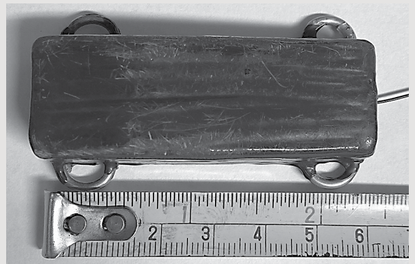
An external GPS transmitter approximately 2.5 inches long
