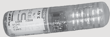
An internal radio transmitter approximately 4 inches long
